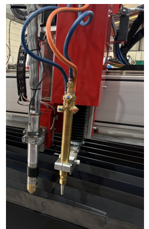
Plasma torch & Oxy-Fuel head mounted on separate torch posts
